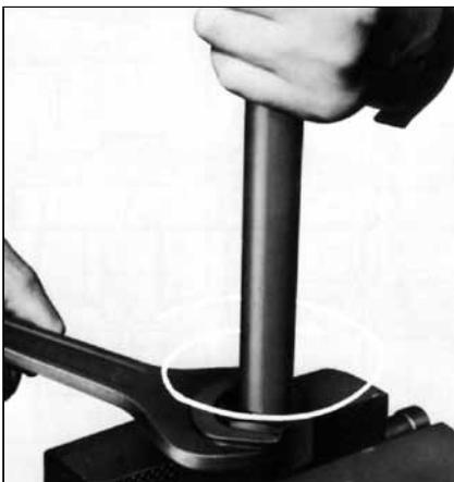
Tighten the nut 1-1/4 turn with a spanner from the grip point.
